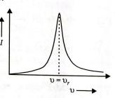
broadcasting stations. To receive one particular radio station/T.V. channel, we tune our receiver set by changing the capacitance of a capacitor in the tuning circuit of the set such that resonance frequency of the circuit becomes equal to the frequency of the desired station. Therefore, resonance occurs. The amplitude of current with the frequency of the signal from the desired station becomes maximum and it is received in our set.
