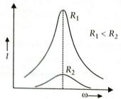
At resonance, when maximum current flows through the circuit.
