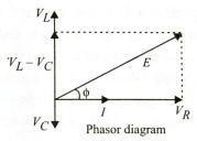
which lags behind current *I* by phase angle of  $\pi/2$ , and voltage drop across the resistor is
