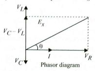
which lags behind current *I* by phase angle of  $\pi/2$ , and voltage drop across the resistor is
