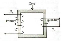
Principle: When the current flowing through the primary coil changes, an emf is induced in the secondary coil due to the change in magnetic flux linked with it *i.e.*, it works on the principle of mutual induction.
