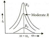
The Q-factor of a series resonant circuit is defined as the ratio of the resonant frequency to the difference in two frequencies taken on both sides of the resonant frequency such that at each
