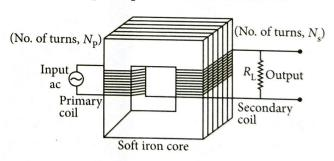
An alternating potential  $(V_p)$  when applied to the primary coil induced an emf in it.
